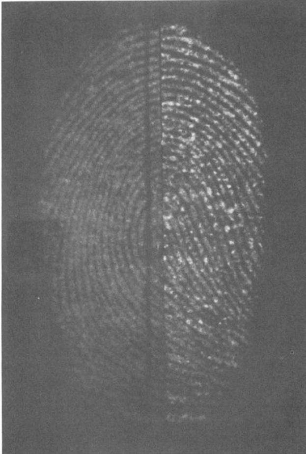
FIG. 3—Latent print under all lines blue-green Ar-laser excitation. Left half treated with ninhydrin/ Cd(NO_3)_2 , right half with ninhydrin/ ZnCl_2 .
